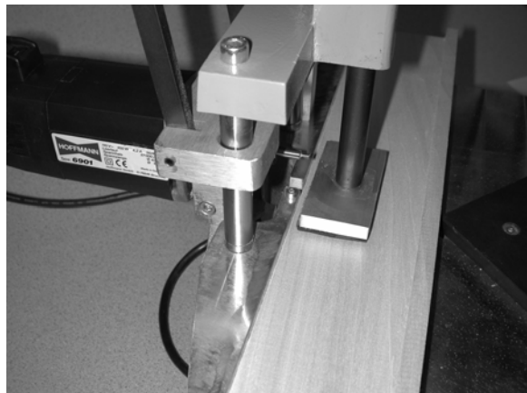
SCRAP WOOD PLACED ON MACHINE TABLE FOR INITIAL CUT THROUGH NEW CHIP BREAKER
