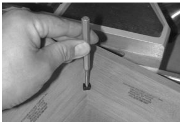
place miter face tight against back fence
