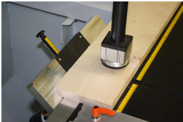
Side panel and assembled face-frame with 45 degree miter on machine table during keyway routing process.
