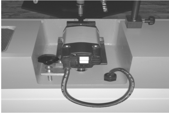
Lift motor carriage with threaded stem
