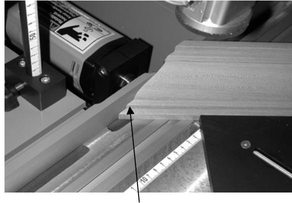
place miter face tight against back fence
