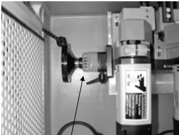
Router spacing adjustment wheel with locking lever and display (PP2-TAB)
