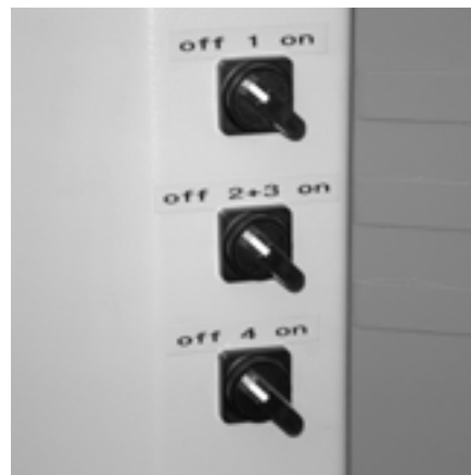
Selector switches for left hand (1), center (2+3) and right hand (4) router head (PP2-TAB/4)
