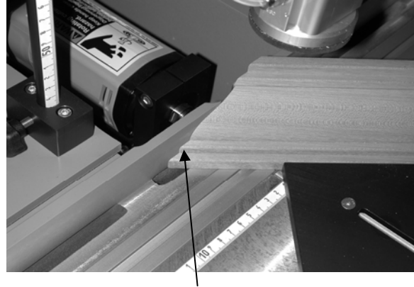
place miter face tight against back fence
