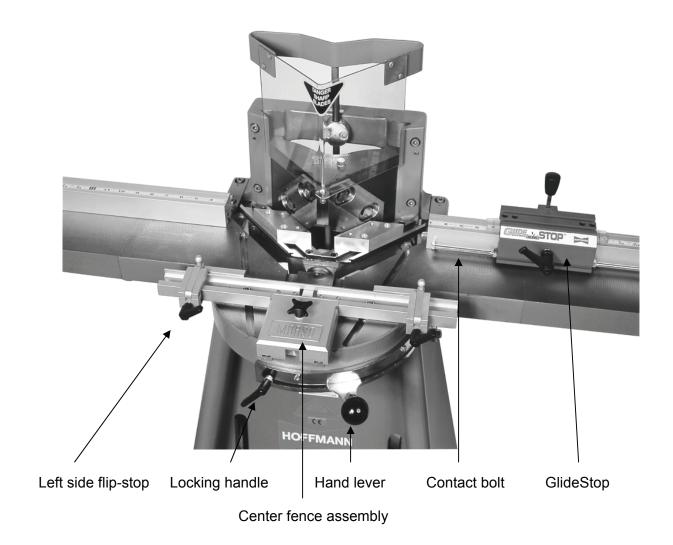
MORSO NFXL manual notching machine with DGS 1000 fence system shown Installation and set-up is identical on MORSO NXLEH electro-hydraulic model.
