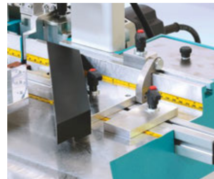
Right side shutter fence plate shown registered against flip-stop
