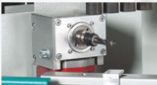
Router motor with 90° gear head
