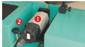
Machine components 1. Router motor 2. Height adjustment
