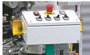
Operator panel with two-hand safety controls
