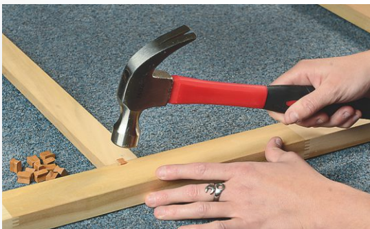
Assembly of strainer cross brace joint
