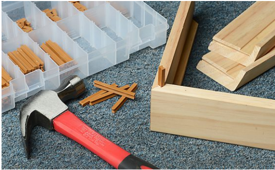
Assembly of shadow box corner joint
