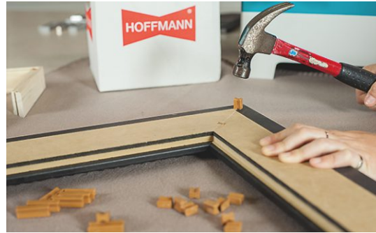
Assembly of wide moulding with two Keys
