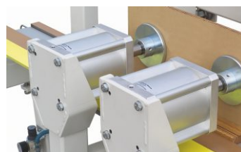
Each station features two horizontal clamping cylinders to secure the panels and two vertical short-stroke cylinders to pull the panels down onto the edgebanding.
