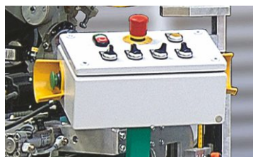
Operator panel with two-hand safety controls
