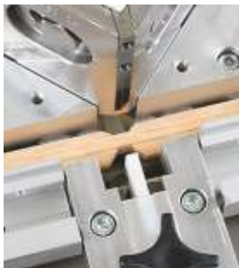
Mullion bars are notched on MORSO notching machine.
