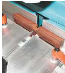
Mullion bars are routed on Hoffmann routing machine.
