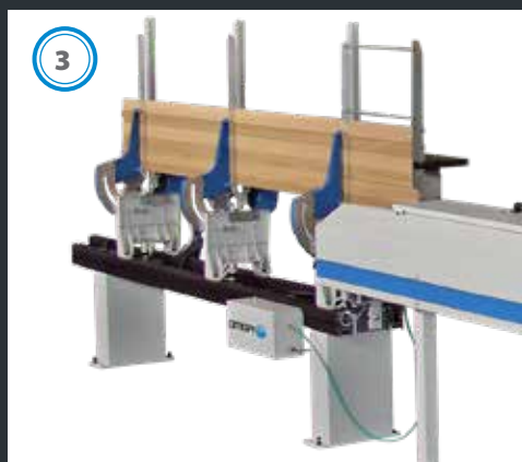
Pneumatic transfer conveyor belt 2000 x 600 mm
